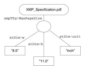
Figure 3 — Example of structure values
